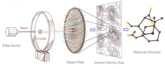
• The process of X-ray crystallography.
